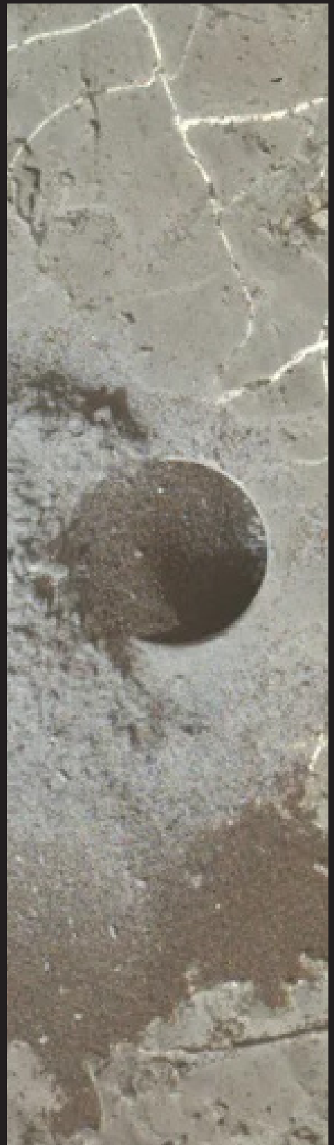
A borehole drilled by Perseverance, The core samples are to be collected and possibly be sent back to earth for examination
